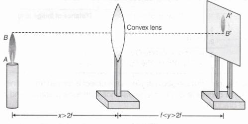
Fig. 2 Formation of image by thin convex lens
