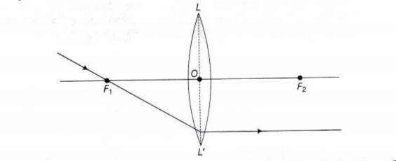
Fig. 2 Refraction by convex lens for a ray passing through a principal focus  $F_1$
