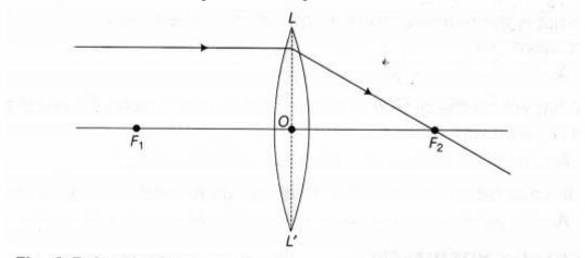
Fig. 1 Refraction by convex lens for a ray parallel to its principal axis
