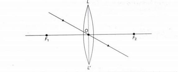
Fig. 3 Refraction by convex lens for a ray passing through the optical centre
