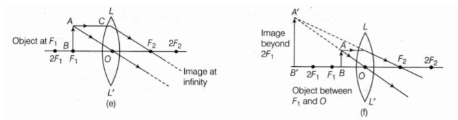
Fig. 6 Ray diagram for each position of the object
