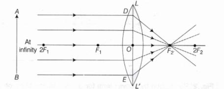
Fig. 5 Formation of image by convex lens for an object at infinity
