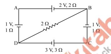
Using Kirchhoff's rules, calculate the potential difference between B and D in the circuit diagram as shown in the figure.
