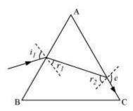
Angle of prism,  $\square A = 60^{\circ}$ Refractive index of the prism,  $\mu = 1.524$
