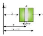
Magnetic flux associated with element dy,  $d\phi = BdA$ Where,
