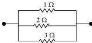
Equivalent resistance of the circuit is given by,
