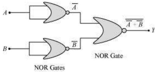
$\bar{A}$  and  $\bar{B}$  are the inputs for the last NOR gate. Hence, the output for the circuit can be written as:
