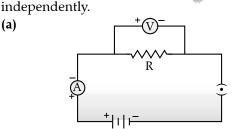
The formula states that the current passing through a conductor is directly proportional to the potential difference across its ends, provided the physical conditions like temperature, density, etc. remain unchanged. This is Ohm's law.
