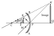
The image is formed behind the mirror. The image is virtual, erect and magnified. 1 + 1 + 1
