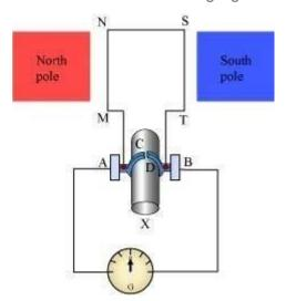
In this arrangement, brush **A** always remains in contact with the length of the coil that is moving up whereas brush **B** always remains in contact with the length that is moving down. The split rings **C** and **D** act as a commutator.
