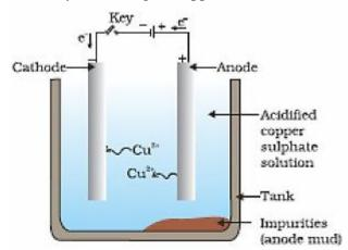
In electrolytic refining of copper, electrolyte is a solution of acidified copper sulphate. Anode is made up of impure copper. Cathode is made up of a strip of pure copper metal.
