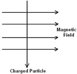
**Solution:** Using Fleming's left hand rule we can easily find out that the nature of the charge on the particle is positive.
