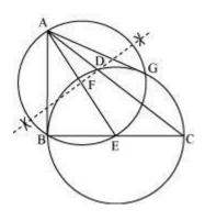
The construction can be justified by proving that AG and AB are the tangents to the circle. For this, join EG.
